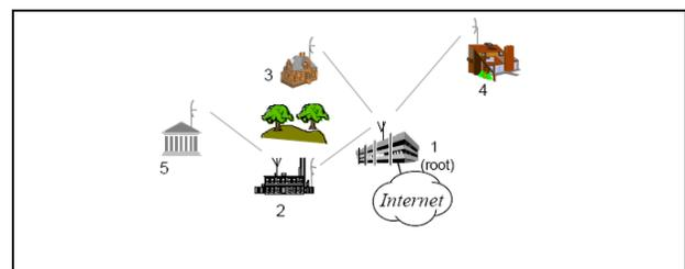
Figure 2. New subscriber with no LOS – Use radio 2 as repeater
