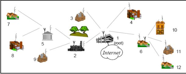
Figure 3. Expanded VINE Network covering large area with no backbone
